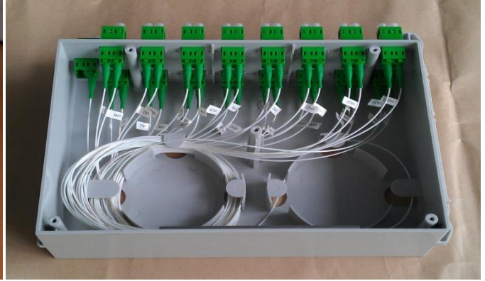
Inner view of 1x32 optical splitter
